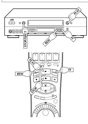
The easiest, most basic operation possible with your video recorder is tape playback. Already-recorded signals on a video tape are read by your video recorder and displayed on your TV just like a TV programme.
